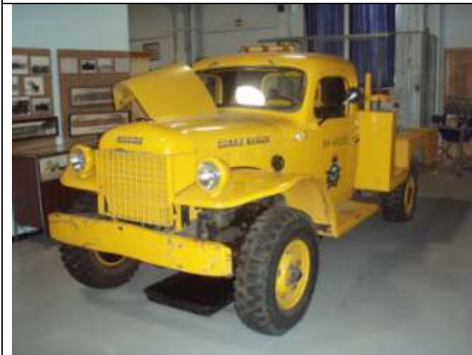
Of special interest to this group a restored yellow 1954 RCAF contract Dodge US made C-1-PW-26 1-ton 4x4 Arc Welding 300 AMP truck! RCAF number 54-69310.
