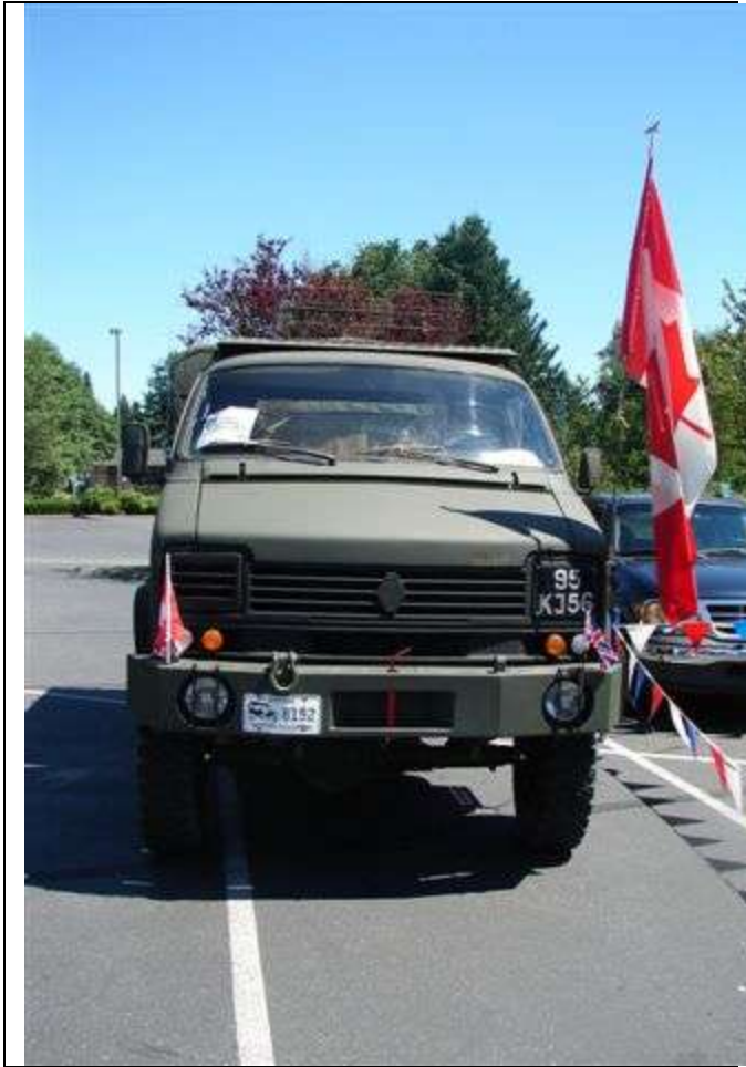
Ian Newby's ex-British Army RB44 number 95 KJ 56. A Reynolds Boughton RB 44 Light Utility Truck
